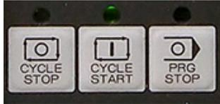
[CYCLE STOP] also called Feed Hold, this will pause motion immediately without completing the current block.
