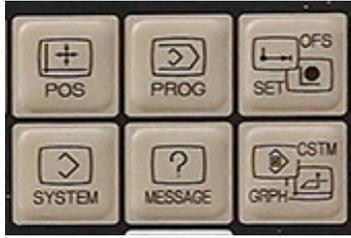
[POS] Stands for position, pressing this will display on the screen the current position with the soft keys offering different coordinate systems. Relative, Absolute, Machine, or Distance To Go.
