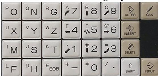
These keys are used to input information first to the input buffer, an editing line at the bottom of the screen. The [INPUT] key is used to copy the text from the input buffer into the control. The most commonly used letters are available, with the less common ones available by first pressing the [SHIFT] key. You do not need to hold down shift, a ^ will be displayed in the input buffer meaning shift is active. [SHIFT] [Z] would put a W in the buffer.
