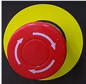
This is a standard twist lock switch. It tells the control to immediately stop all motion, including the spindle and all axis. Always depress this switch prior to turning the main power switch on or off as a safety measure.
