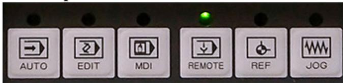
Similar to the display modes, however these change which input will control machine motion. Only one switch can be active at any time and they must be chosen correctly for the desired function to be performed both by the
