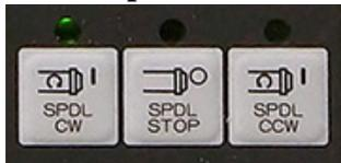
[SPDL CW] turns the spindle on at the last programmed speed, can only be used in JOG mode. **Must be used to re-start the spindle if you stopped the spindle during regular operation.**
