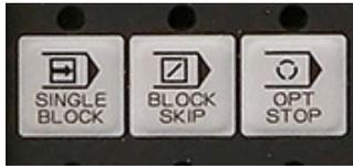
[SINGLE BLOCK] stops the control after executing each line of code
