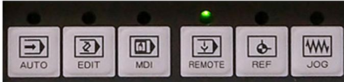
Similar to the display modes, however these change which input will control machine motion. Only one switch can be active at any time and they must be chosen correctly for the desired function to be performed both by the
