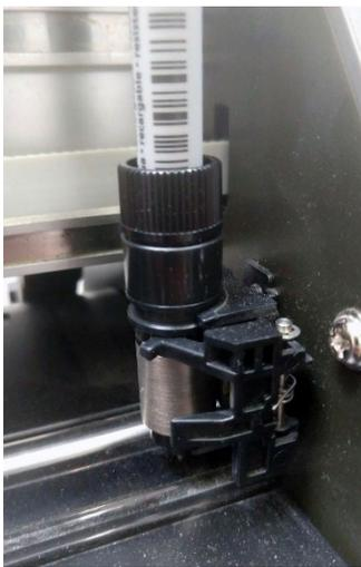
Next, take the pen out of the height gauge and place it into the holder on the right of the machine. Gently pull the spring loaded foot toward you and slide the collet into the holder. Do this while the machine is off. Ensure that the pen is located EXACTLY as in the image to the left, with the top channel fitting into the semicircular holder and the spring clip grabbing onto the lower channel.
